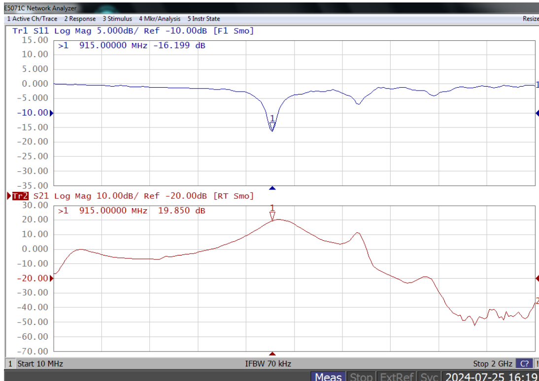
Figure 6: Network analyzer output, S11 and S21
