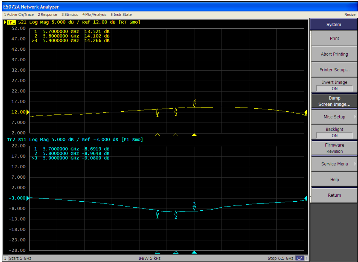
Figure 4: S11/S21 output from Network analyser (VDS= 50V, IDQ=200 mA Vgs =-3.0V)
